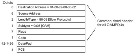
Figure 57-9—OAMPDU frame structure
